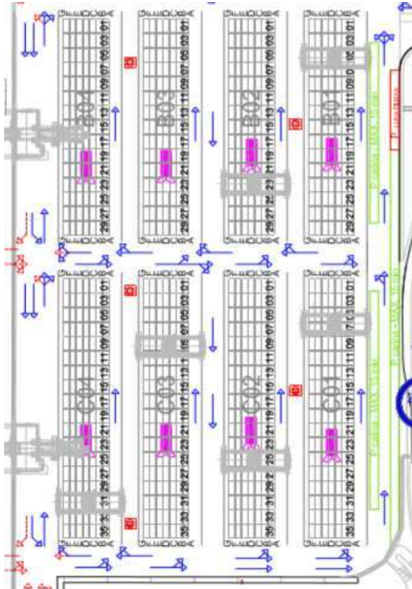
Figure 4: Storage area SA2 with RTG cranes Source: AGCT, 2020.
