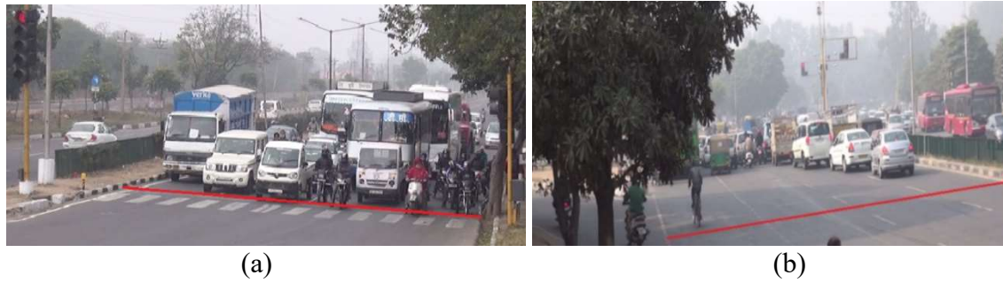
Figure 1: Formation of trap from (a) stop line to (b) end of the queue at study locations
