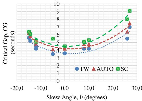
Figure 5: Critical Gap for Minor TH.
