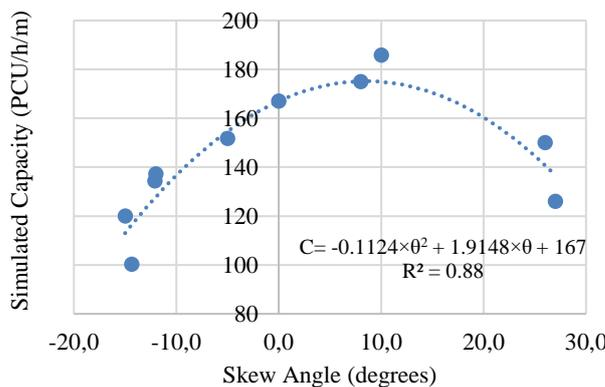
Figure 12. Capacity Model for Minor TH.
