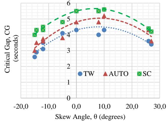
Figure 4: Critical Gap for Minor RT.
