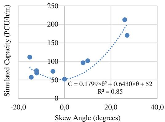
Figure 10: Capacity Model for Major RT. Figure 11: Capacity Model for Minor RT.
