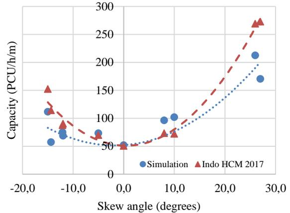
Figure 8: Capacity for Minor RT.
