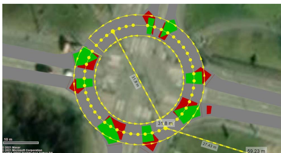
Figure 10: Design of the southern roundabout
