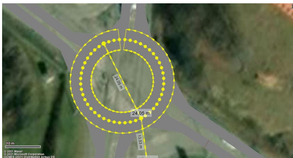
Figure 11: Design of the northern roundabout
