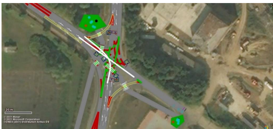
Figure 6: The progress curves and their crossing required for determining the first intermediate time interpreted in the model
